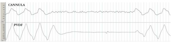
In both test cases, visual inspection of the response waveform characteristics of PVDF output compared to nasal pressure output showed similar traces throughout the test period. Peaks and valleys seen in the traces, as well as flattening of the signal during apnea, were near synchronous between the two methods, indicating that response times between the two methods are similar.
