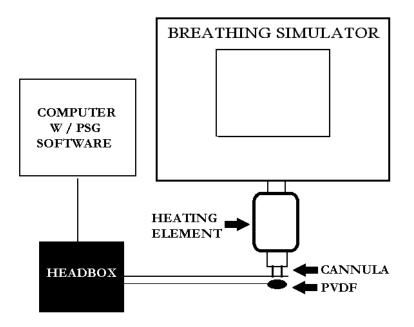
With the test setup and PSG software operational, and the heating element set to "off", the sleeping breathing pattern was initiated. Data was automatically recorded by the PSG software. A second test was then run, with the heating element set to "on" and at the minimum available setting. On completion of the breathing simulations, data was extracted and screenshots of the nasal pressure and PVDF traces over the 2-minute simulated breathing period were taken.
