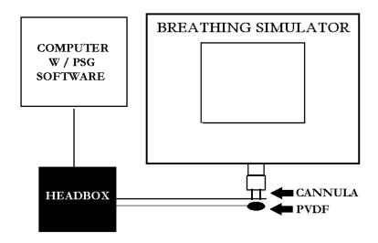
With the test setup and PSG software operational, the Normal breathing pattern programmed in the simulator was initiated. Data was automatically recorded by the PSG software for up to five minutes. Similarly, each of the Apnea and Hypopnea patterns was run and data recorded by the PSG software. On completion of the breathing simulations, data was extracted and screenshots of the nasal pressure and PVDF traces over a 2minute period were taken.
